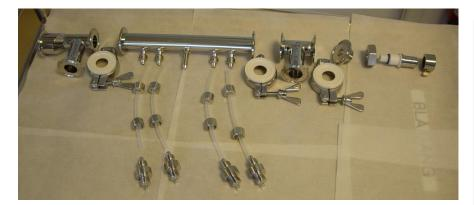
Tubing cut, washed, dried, connected and sterilised in house.
